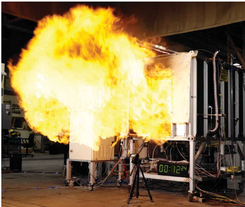
To learn how firefighters could anticipate deadly backdraft events in the field, NIST researchers conducted hundreds of fire experiments while taking a plethora of measurements. Many of these tests resulted in a backdraft, which caused fireballs to burst from the opening of a metal chamber. Credit: D Stewart/NIST
